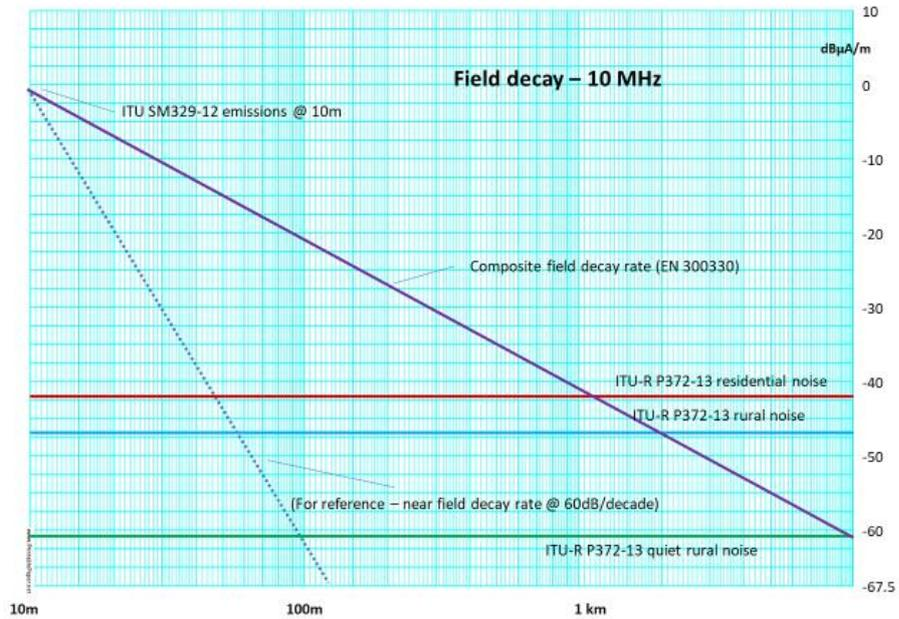
Figure 3b: Decay rate of emissions with distance at 10 MHz
