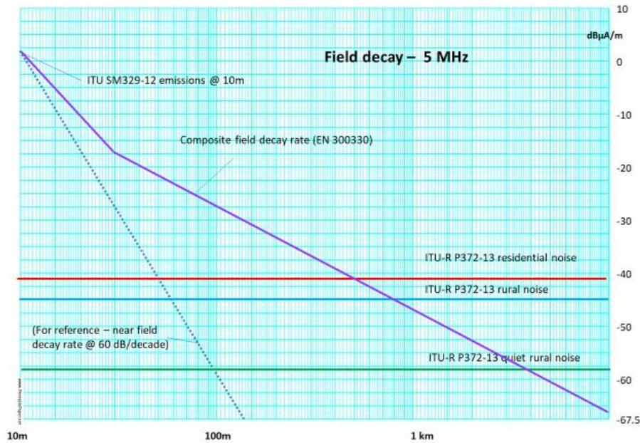
Figure 3a: Decay rate of emissions with distance at 5MHz
