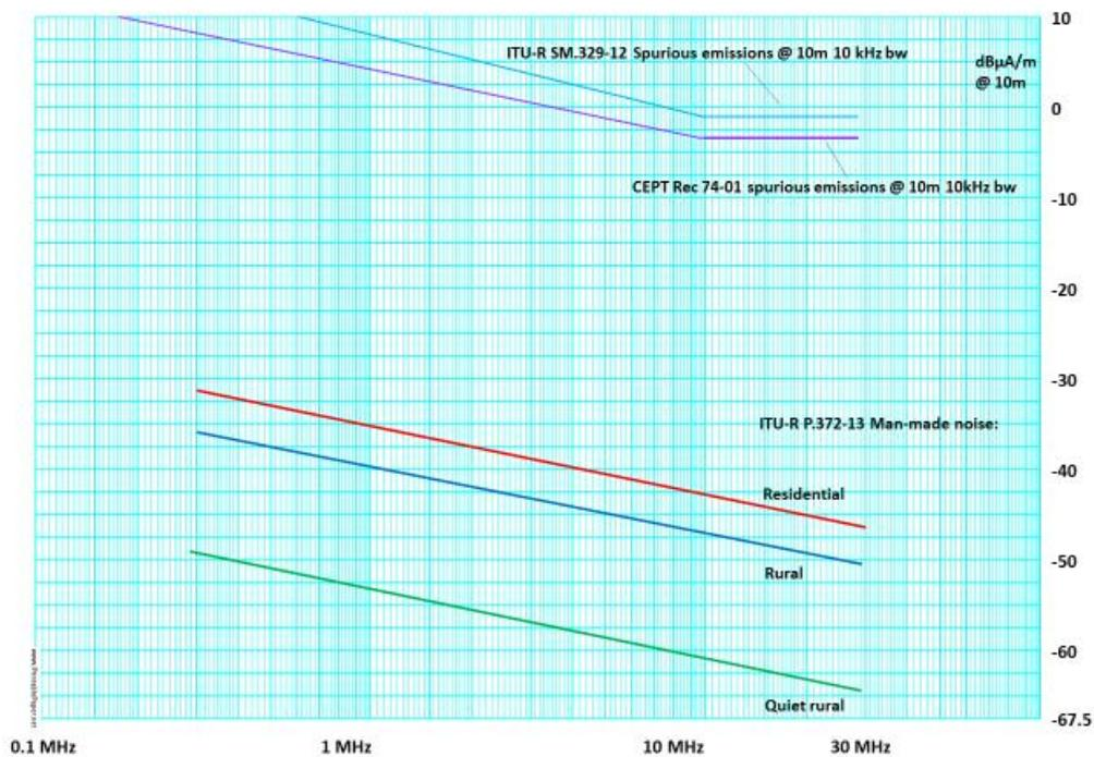
**Figure 2: Graphical representation of the current spurious emission limits compared with background noise levels in ITU-R P.372-13**
