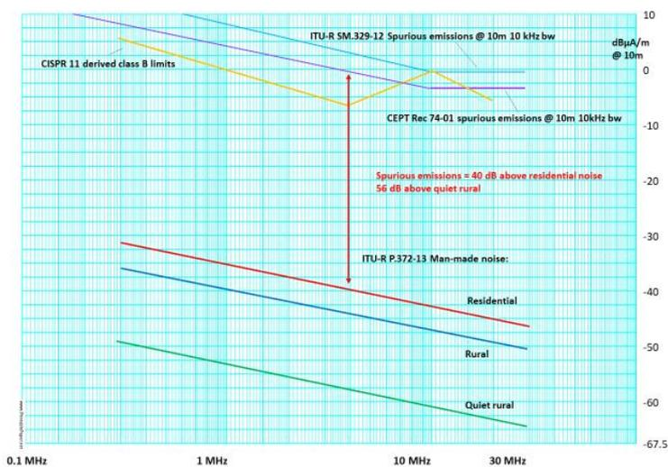
Fig 5 ERC 74-01, ITU-R SM.329-12 and CISPR 11 compared to ITU-R P.372-13 noise levels
